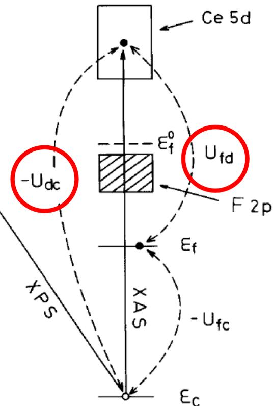
Fig. 1. Model of the present theory describing 3d-XPS and L<sub>3</sub>-XAS.
